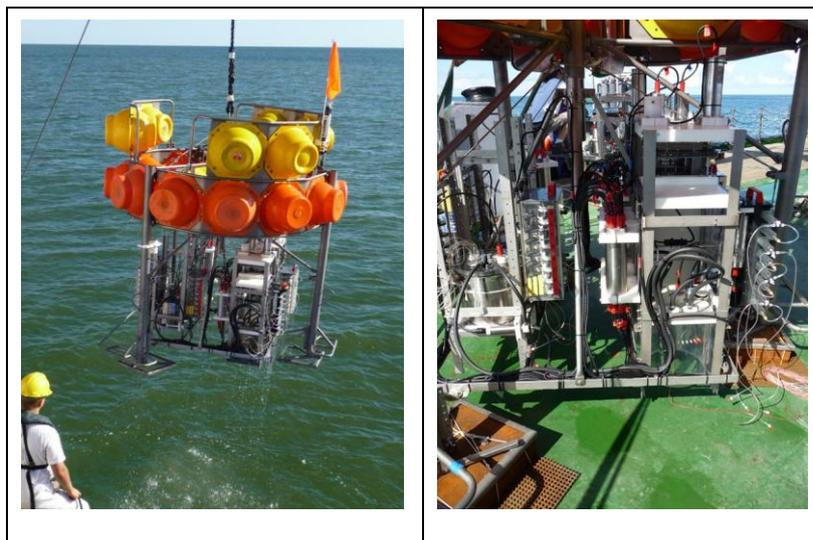
A new micro-electrode sediment profiler which was developed at IFM-GEOMAR in cooperation with Unisense (Arhus,DK) was successfully deployed down to 1000m integrated into a GEOMAR Modular Lander (Fig. 2). The profiler module can also be placed with a ROV on the sea floor. The new profiler has unlike its predecessors the capability to measure in three dimensions (x/y/z). The profiler unit carries four micro-electrodes which can measure oxygen, H<sub>2</sub>S and pH.
